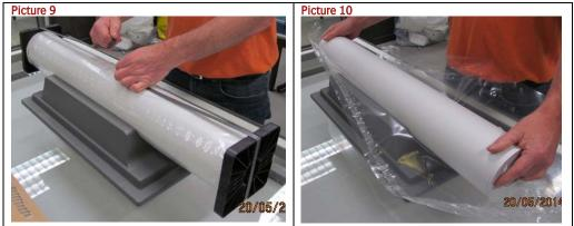
Remove the strap and the transport flanges (picture 9). Remove the plastic anti dust wrapper (picture 10).
