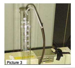
4. Hook the replenishment pipe in a 500 ml measuring glass to enable accurate readings (see picture 3). Make sure the replenishment tank is at least half full. If not it might be impossible to pump up the required quantity.
