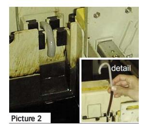
3. Take out the plastic pipe from this fitting and lift it up. (see picture 2)
