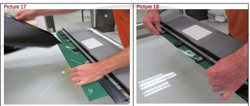
Sepparate the leader from the film (picture 16 and 17). Rewind manually and position the film into the loading position: in line with the front side of the cassette (picture 18).
