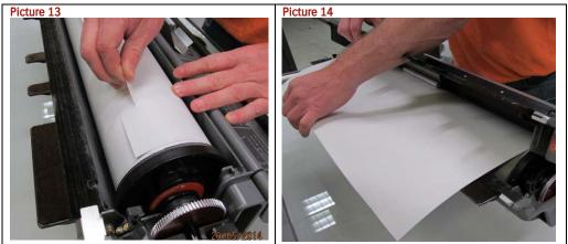
Remove the tape that secures the filmleader (picture 13). Pull the leader approximately 15 cm over the edge of the cassette and close it (picture 14).
