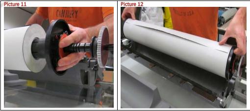
Mount the endcaps of the supply cassette onto the roll core (picture 11). Place the roll with mounted endcaps in the supply cassette (picture 12).
